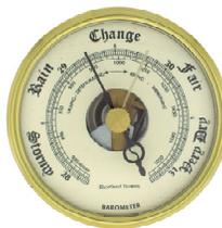
**A barometer** measures air pressure. The atmosphere has weight, and thus exerts pressure. A barometer is the instrument that measure the amount of pressure the atmosphere is exerting over a location.
