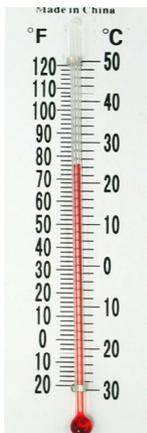
A thermometer is used to measure temperature. The word thermometer is a combination of “thermo,” which means heat, and “meter,” which means to measure. The thermometers we commonly use are called bulb thermometers. They are usually filled with mercury, a mineral that is liquid at room temperature.
